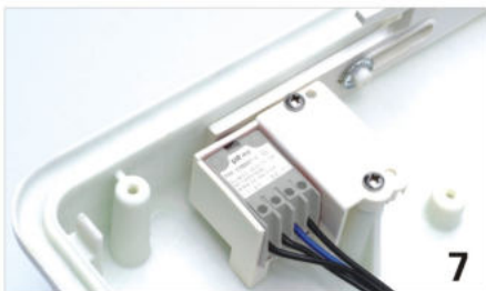
Ex de IIC 防爆行程开关模块由联锁机构进行操作，当开关处于分断时壳体才能打开 The explosion-proof isolation switch module of Ex de IIC is operated by interlocking device and the enclosure can only be opened when the switch is off.
