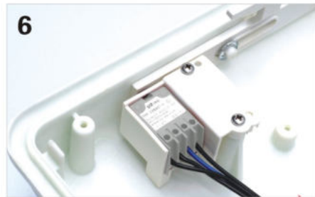
Ex de II C 防爆行程开关模块由联锁机构进行操 作，当开关处于分断时壳体才能打开 The explosion-proof isolation switch module of Ex de IIC is operated by interlocking device and the enclosure can only be opened when the switch is off.
