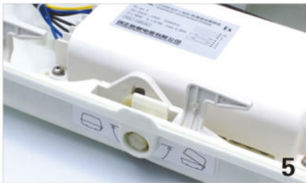
开锁装置通过联锁机构将壳体与透明罩使其压紧并带动防爆行程开关的分断联锁功能 The enclosure and transparent shield are pressed tightly and drive the switching off and interlocking function of explosion-proof isolation switch by unlocking device through interlocking mechanism.
